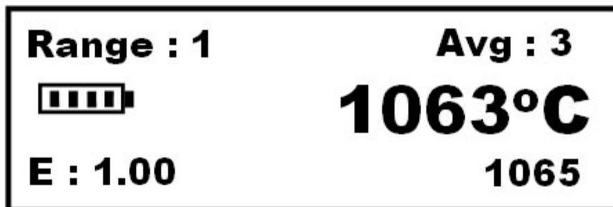
The large characters display the present temperature. The smaller numerals in the lower right portion of the screen display the average of the measurements made while pushing the average button.
