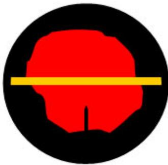
**B. 2. The lamp current is raised until the filament becomes hotter than the target and it appears brighter than the target.**
