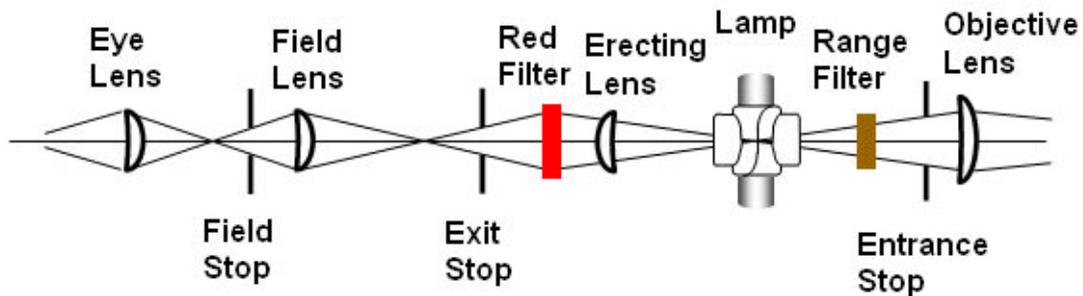
**B. 1. The lamp filament is initially cooler than the target and appears dark before it. The sighting index appears black below the filament.**
